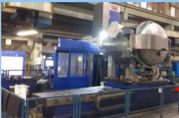
The machining of spacious parts on a WHN boring machine e.g : machine bodies, plates with high grade accuracy. The weight of a single part is up to 12 ton
